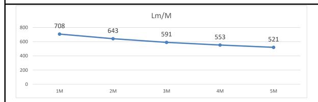
From above chart, please connect 5M at most by one-end power to keep brightness consistency.
