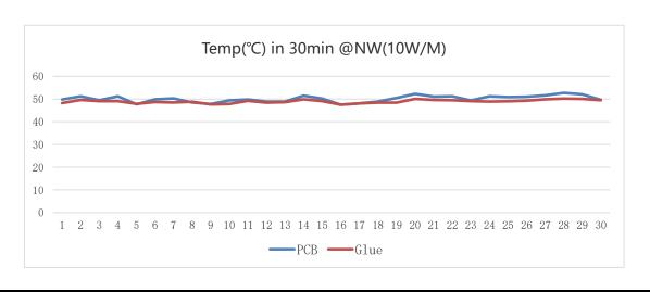
The above curves indicate the temp. changing in glue, & PCB within 30 minutes after powering on, under the ambient temperature of 25  $^{\circ}$ C.
