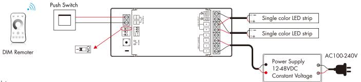
The maximum current of each terminal is 10A, when the input voltage is 12/24V and the working current is more than 10A, the two positive terminal ports and two negative terminal ports of the power input, the LED output two positive ports must be wired at the same time, otherwise the current will cause the risk of burning the wiring port.
