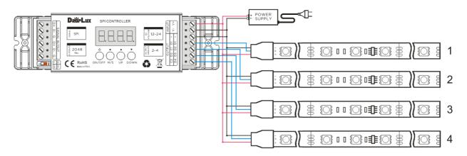
2) Diagram with double-signal-wire digital led strip (such as: LPD6803)
